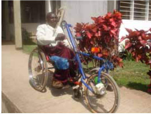
Figure: Examples of tricycle attachments from Sri Lanka attached to a 3-wheeler in Tanzania and front adaptor attached to a traditional hospital wheelchair in Zimbabwe
