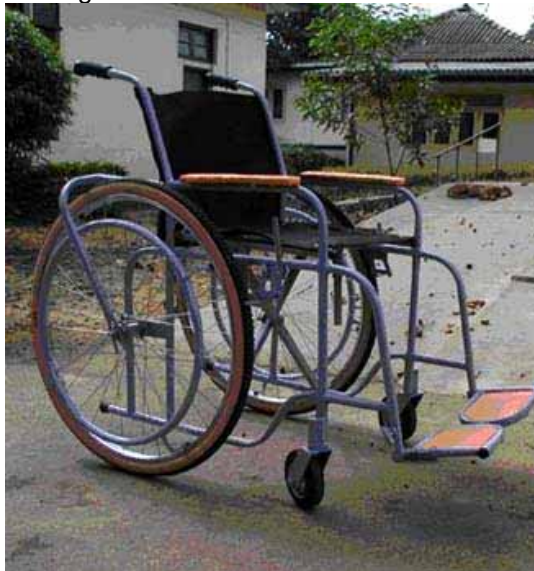
Example of wheelchair design that was tested and failed the strength tests
