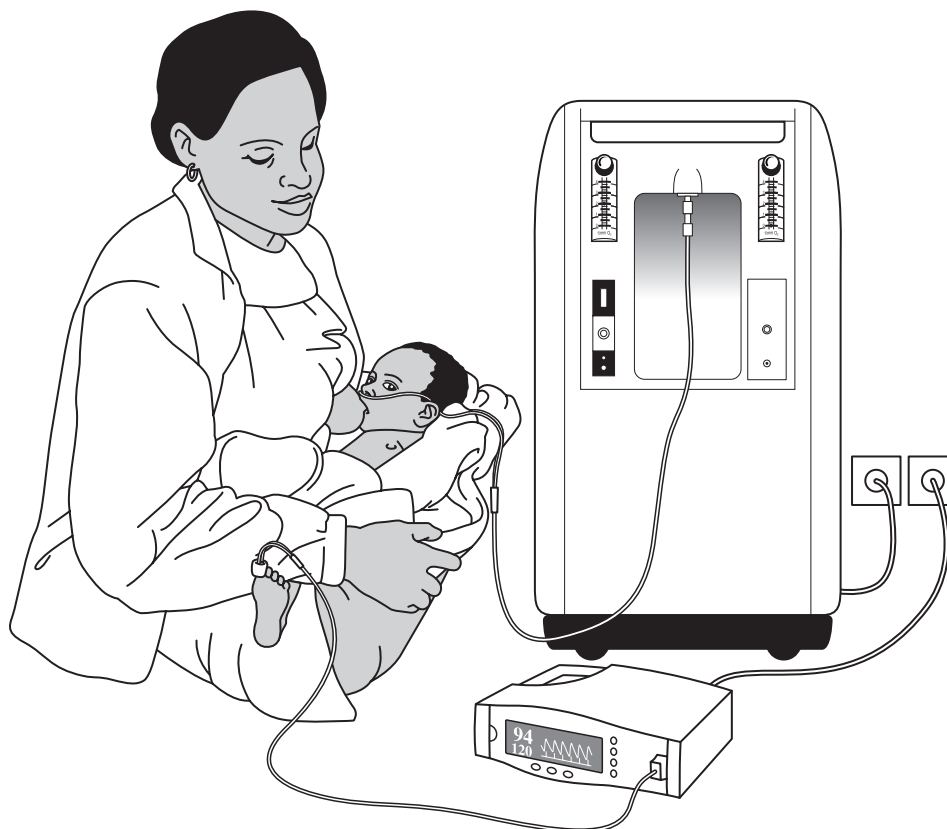
Figure 2. Setup of a typical oxygen concentrator, pulse oximeter and connection to the patient
