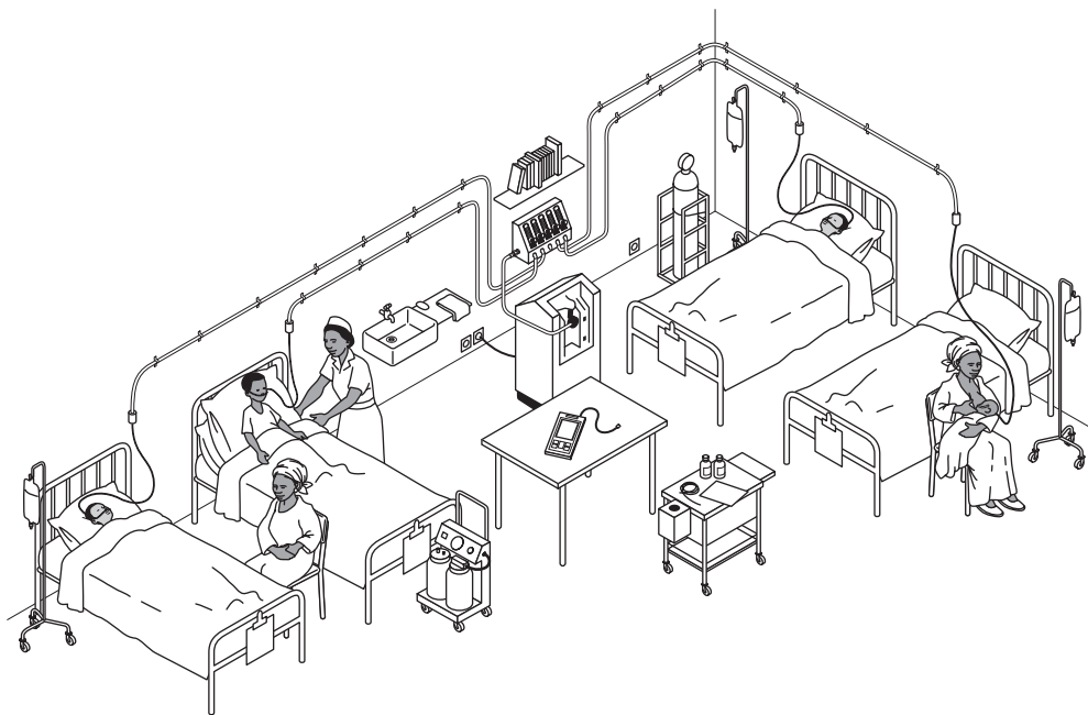
Figure 8. Example setup of an oxygen concentrator in a paediatric ward
